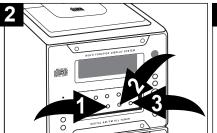
Press the TUNING/CD SKIP/ SEARCH (►►) ① or (►<) ② button to set the hour, then press the MEMORY/TIME SET button ③ again; the minute digits will blink. Press the TUNING/CD SKIP/SEARCH (►►) ① or (►<) ② button to set the minutes, then press the MEMORY/TIME SET button ③ again.
